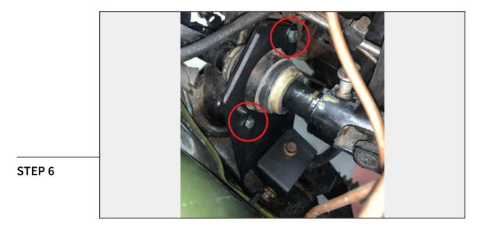
Secure the bearing to the bracket using (2) M6 bolts and the original (2) 10mm nuts. Tighten all hardware until secure.
