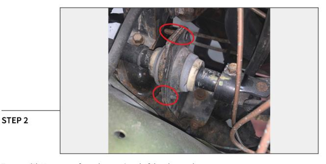
Remove (2) 10mm nuts from the steering shaft bracket studs.
