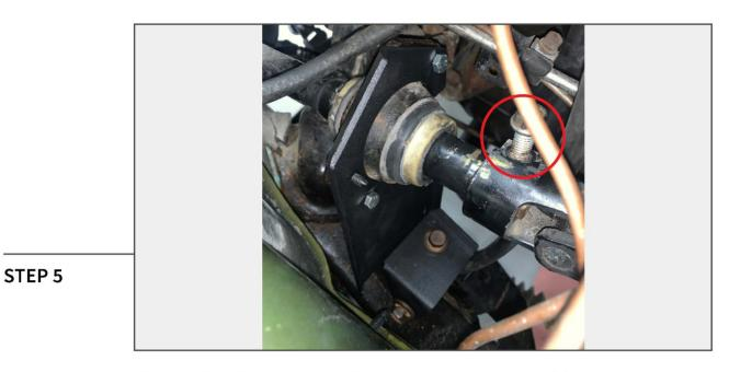
Insert the intermediate shaft to the steering shaft, secure using the original (1) 13mm bolt.
