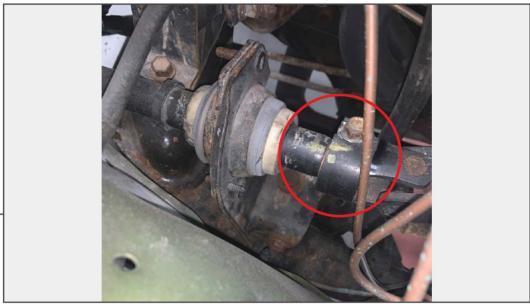
Loosen (1) 13mm bolt securing the steering shaft to the intermediate shaft. Separate the two steering shafts. Remove the (2) 15mm bolts from Step 1, and remove the original steering shaft
