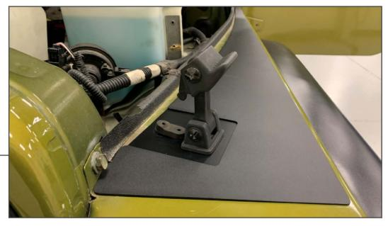
Install the hood latch to the vehicle reusing the original hardware.
