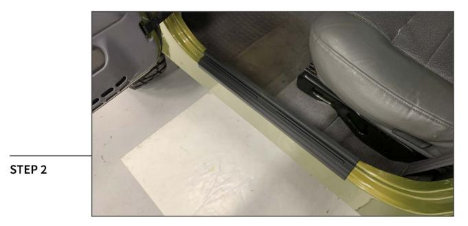
Peel the red tape backing from the double sided tape. Firmly press the door sill plate to the vehicle.
