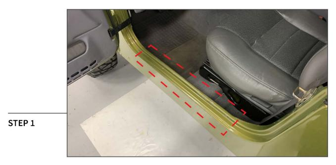
Clean the door sill area of the vehicle using isopropyl alcohol and a microfiber cloth. After cleaning, ensure the area is dry.
