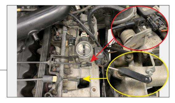
Disconnect the linkages from the throttle body.
