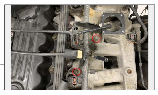
Remove (3) bolts from the linkage bracket.
