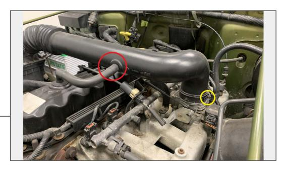
Disconnect the PCV hose from the intake tube. Loosen the hose clamp connecting the intake tube to the throttle body. Lift the intake tube from the throttle body and temporarily relocate tube towards the vehicle firewall.
