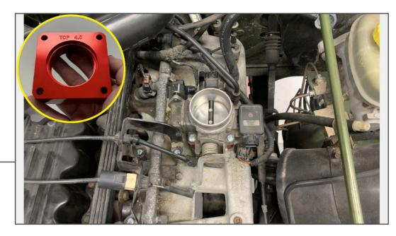
Place (1) throttle body gasket between the intake manifold and the throttle body spacer. Then, place (1) throttle body gasket between the throttle body spacer and the throttle body. Secure the throttle body & spacer to the vehicle using (4) M6 x 50mm bolts and (4) M6 flat washers. Tighten until secure.
