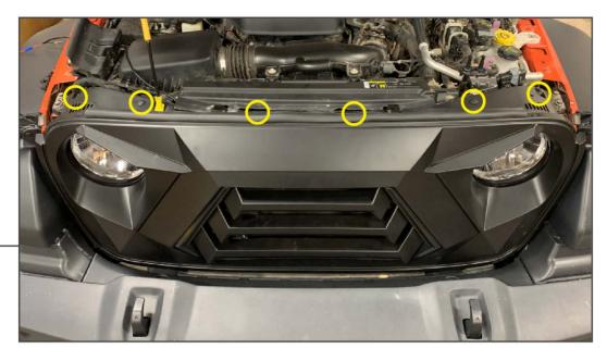
Align the top of the grille to the radiator support and secure into place using the provided (6) push clips.
