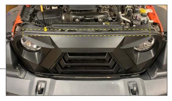
Clean the upper portion of the grille using isopropyl alcohol and a microfiber cloth. Adhere the weatherstrip to the top of the grille. Close the hood.
