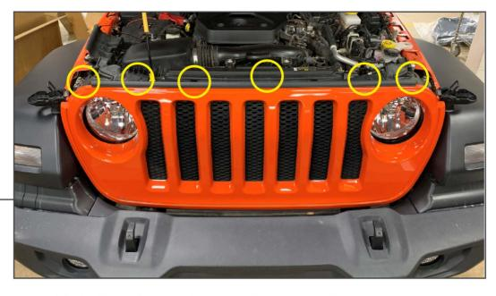
Open the hood. Remove (6) plastic push clips using a panel removal tool.
