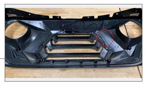
Clean the designated area of the grille using isopropyl alcohol and a microfiber cloth. Adhere the DRL harness module to the back of the grille.
