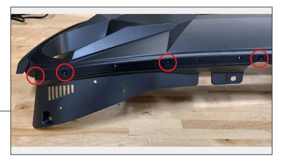
Install each backing panel to the new grille using the provided (4) tree clips per panel.
