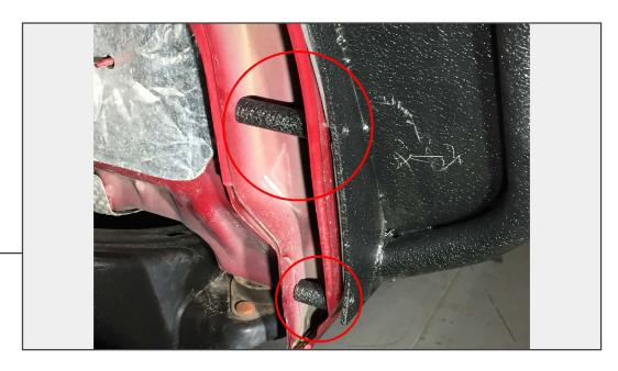
Install the supplied spacers between the inner and outer fenders using the M8 x 1.25 120mm bolt for the long spacer and the M8 x 1.25 65mm bolt for the shorter spacer.
