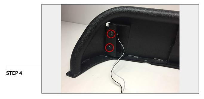
Mount the light/light bracket assembly to the fender using the supplied Allen bolts and washers.
