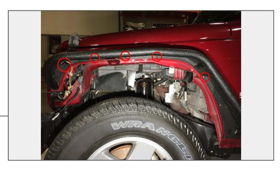
Install the flares to the vehicle using the supplied M8 x 1.25 25mm long Allen bolts, install the forward most (5) bolts first. Loosely install all hardware before fully tightening bolts to ensure proper bolt hole alignment.
