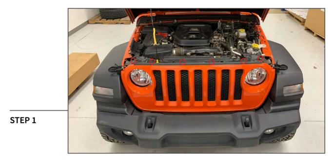
Begin by opening and supporting the hood. Use a soft pry tool to remove the (6) plastic push pins across the top of the grille. Then Firmly pull the grille away from the vehicle. Set the grille aside for re installation later.
