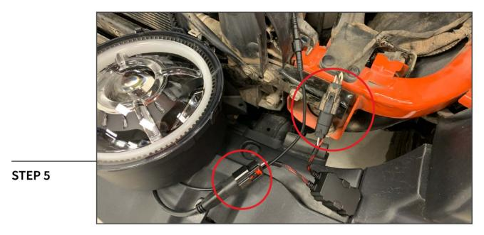
Plug the headlight harness into the vehicle and then into the headlight. Using the factory hard-ware, reinstall the headlights.
