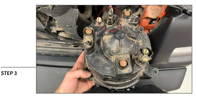
Pull the headlight away from the vehicle. Pull back the red locking tab, then depress the clip and pull the plug away from the light. Remove the light from the vehicle.
