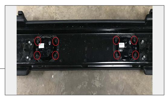
Remove the fog lights from the original bumper by removing (8) Phillips head screws.
