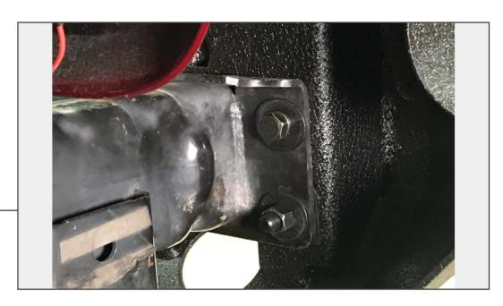
Once the bumper is attached loosely with the nuts, using (4) M12x1.75 x 35mm bolts, (4) M12 lock washers, and (4) M12 flat washers, thread the bolts into the welded nuts on each of the previously installed brackets. Once the bolts are loosely attached, make sure bumper is level on vehicle, and tighten the nuts and bolts to the vehicle using a 18mm socket.
