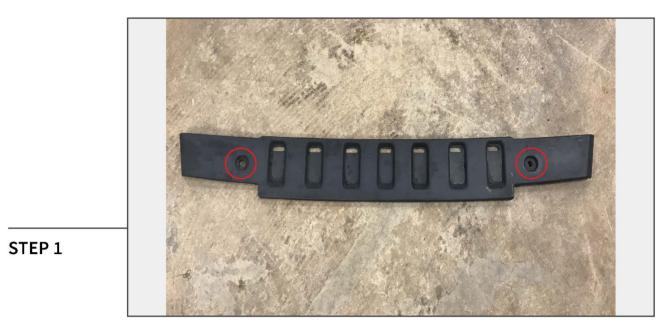
Begin by removing the plastic sway bar cover by removing (2) plastic push clips.
