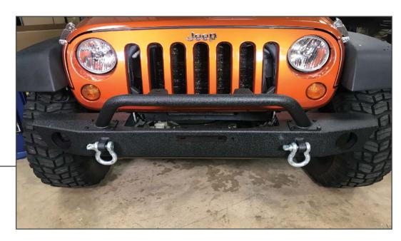
Install the 3/4" D-Rings into the front of the bumper.
