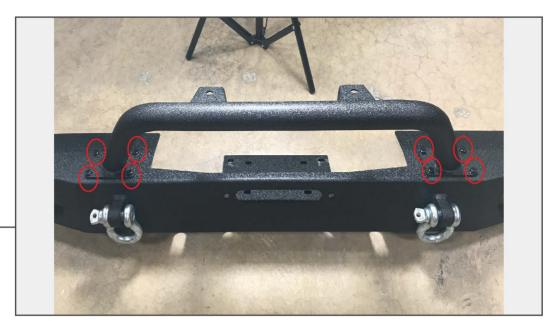
Install the overrider hoop onto the bumper using (8) M8x1.25 x 25mm bolts, (16) M8 flat washers, and (8) M8 nuts. Tighten the nuts and bolts using a 13mm socket and wrench.
