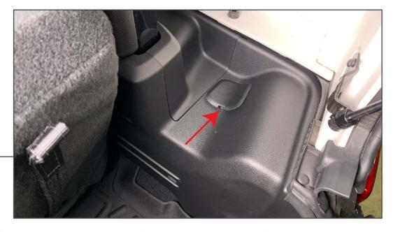
Open the vehicle cargo area to access the tail light trim cover. Using a soft pry tool remove the cover from the vehicle.
