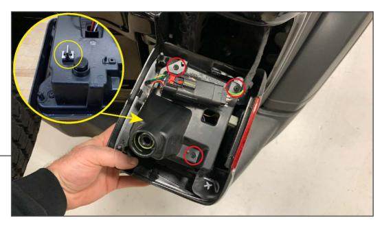
Remove (3) Phillips screws to remove the mounting bracket from the original tail light. Install (1) vampire clip to the stud on the new tail light. Install the mounting bracket to the new tail light reusing original hardware.
