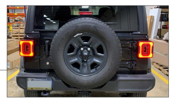
Re-install the new LED tail lights following Steps 1-6 in reverse order. \*\*Note: Vehicles with Blind-Spot Detection will need to transfer the factory tail light sensors from the original light to the new LED light in order to retain Blind-Spot Detection functionality.
