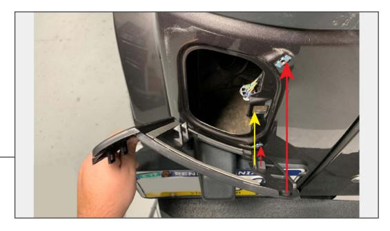
Align the alignment tab in the tail light bracket to the vehicle, then push the panel inwards to lock the outer tabs into place. Ensure the (2) bolt holes remain aligned with the vehicle. Once properly aligned, press the tail light bracket into the vehicle to adhere the tape to the vehicle body panel.
