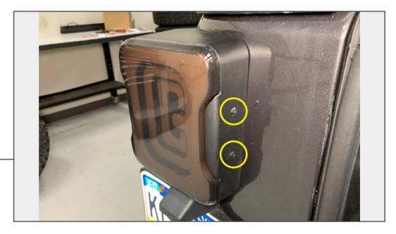
Align the tail light to the tail light bracket on the vehicle. Secure the tail light into place using (2) small Phillips screws.
