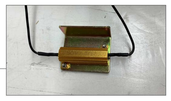
Mount the resistor to the resistor bracket using the supplied M4 hardware. Hold the M4 nut with pliers while tightening the bolt using a Phillips head screwdriver.
