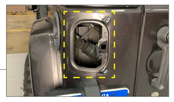
Clean the tail light mounting area of the vehicle using (1) alcohol prep pad.
