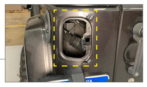
Clean the tail light mounting area of the vehicle using exterior detailer and a microfiber cloth.
