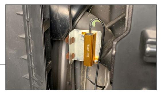
Using (2) 'S' clips per bracket, clip the resistor bracket to the vehicle. Plug the vehicle tail light wiring harness into the new tail light.
