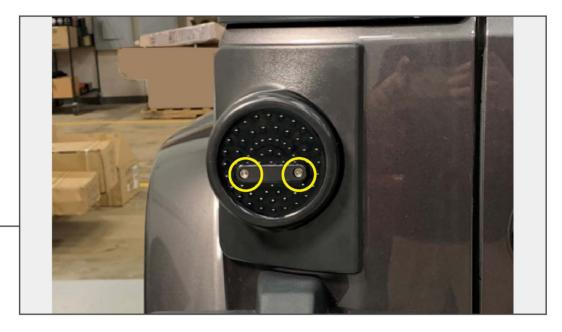
With the bracket properly aligned within the quarter panel, tighten the (2) Allen bolts to secure the tail light into place.
