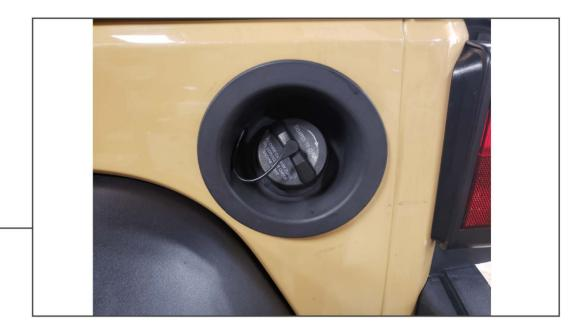
Start by turning the gas cap counter-clockwise to remove from the filler neck.
