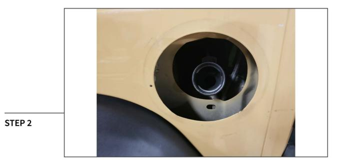
Using a trim panel removal tool, carefully pry around the edges of the factory fuel bezel to release the clips securing it in place. Then pry the rubber gasket around the filler neck and pull away removing the bezel from the vehicle.
