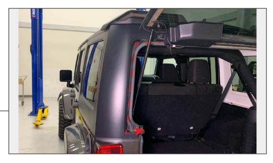
Route the tail light wiring down the side of the hard top channel towards the tailgate. Route the wiring under the seal and towards the vehicle tail light assembly. Use the included wire holders and wire holder adhesive pads to secure the harness to the hard top channel.
