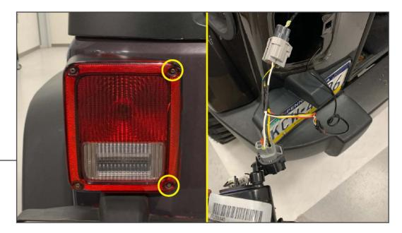
Remove (2) Phillips head screws to remove the vehicle tail light assembly from the vehicle. Once removed, unplug the tail light assembly. Install the included in-line adapter harness to the vehicle wiring harness and the tail light assembly. Plug in the roof mounted tail light.
