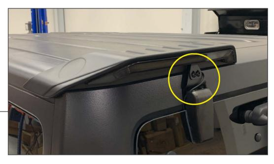
Align the tail light to the roof of the vehicle, ensuring the two previously installed brackets align. Once fitment is confirmed, remove the tail light from the vehicle to prepare for adhering the housing to the vehicle.
