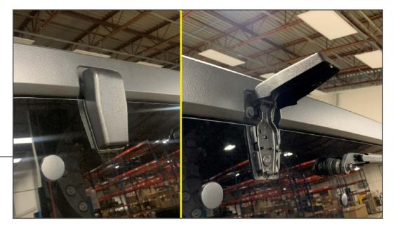
Using a plastic pry tool, gently pry the hinge covers from the rear glass hinges, starting from the bottom. The cover will hinge upward once dislodged. Remove the hinge cover from the vehicle.
