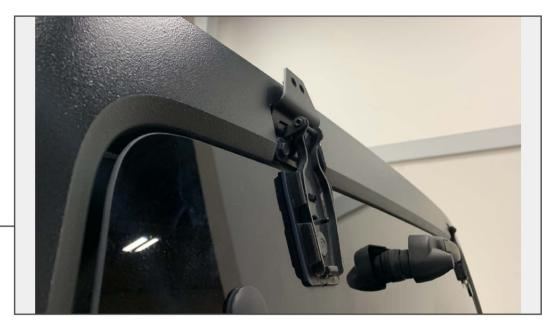
With the bolts removed, place (1) hinge bracket in between the rear glass hinge and the vehicle hard top. Re-install the vehicle hinge to the vehicle.
