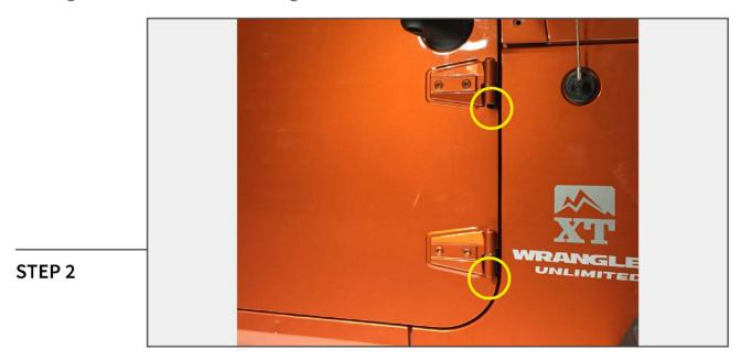
Locate the vehicle door hinge brackets. Remove (2) T-50 Torx hinge nuts to allow the door to be removed.
