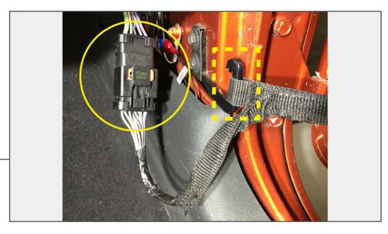
Locate the door wiring harness. Slide the red locking tab outward, then depress the black tab on the connector to release the electrical connection. Once disconnected, lift the door strap over the retaining hook.
