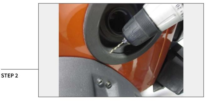
Remove the fuel door from the vehicle and drill the four marked spots with a 7/64 bit as shown.
