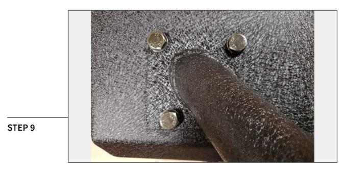
Install the optional over-rider light bar mount, or the (2) block off plates to the bumper by using the (6) M10 x 1.50 x 25mm bolts, (12) M10 flat washers, (6) M10 lock washers, and (6) M10 nuts.
