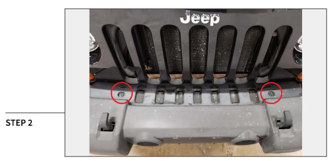
Remove (2) plastic push clips from the upper bumper plastic cover.
