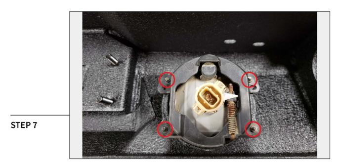
Secure each fog light into the bumper using (4) M4 x 0.7 15mm bolts, (4) M4 lock washers, (8) M4 flat washers, and (4) M4 nuts.
