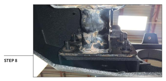
Install the bumper to the frame of the vehicle using (4) M10 x 35mm bolts, (4) M10 nuts, (8) M10 lock washers, and (8) M10 flat washers. Torque the hardware to 40 ft. lbs.
