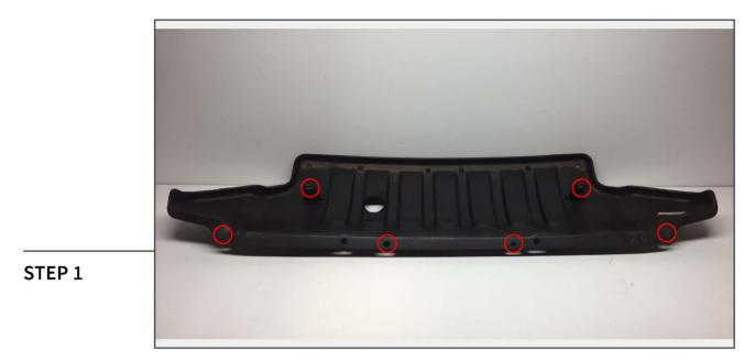
Remove the (6) plastic push pins securing the factory lower splash shield to the vehicle.
