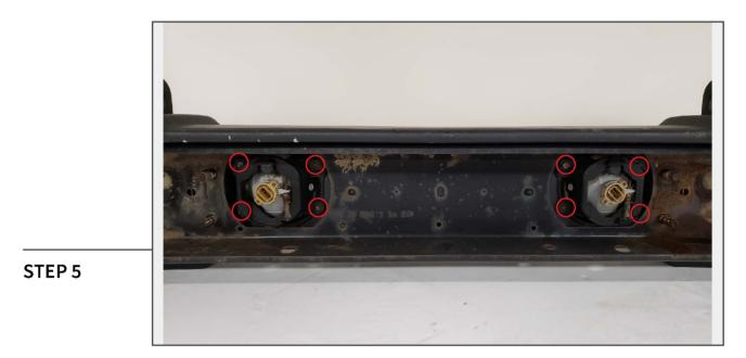
Remove the fog lights from the bumper by removing (8) Phillips screws.
