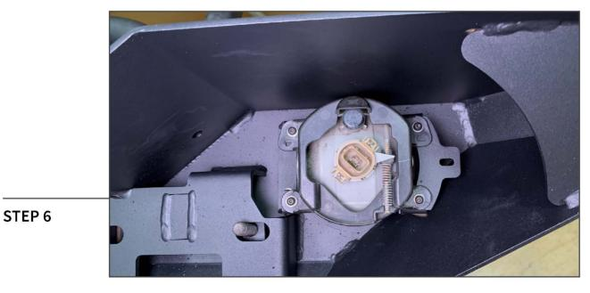
Using (4) M4 Allen bolts, (4) M4 lock washers, (8) M4 flat washers, (4) M4 nuts, attach the fog light to the bumper and bracket installed in Step 5. Repeat for both fog lights.
