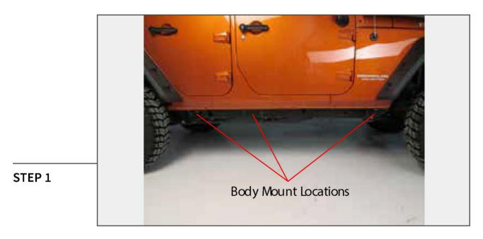
Begin by locating the (3) body mounts that run along the frame of the vehicle.
