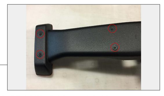
Remove the factory 3rd brake light from the factory tire carrier bracket.
