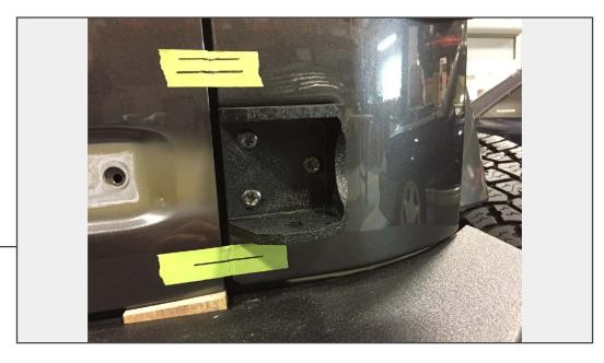
Attach the supplied hinge mounts using the factory T-50 Torx bolts. Tighten the bolts down in triangular pattern, tightening each bolt a little each time, and the hinge will self center.
