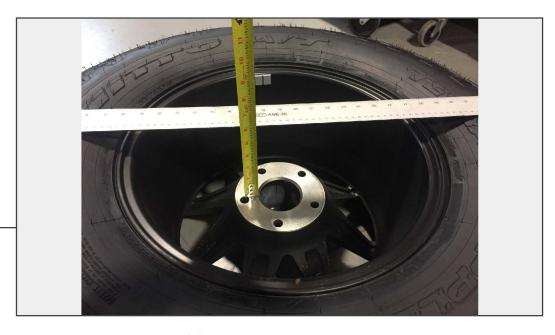
Next, loosely install the tire mount with the (3) threaded studs. The location of the mount will need to be measured and adjusted depending on the backspacing of your wheel and tire. Measure the backspacing by placing a straight edge across the tire. Then, measure to the mounting hub of the tire.
