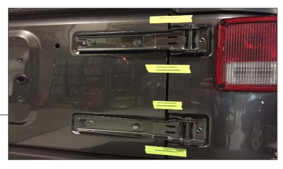
Apply painters tape across the parting line between the tailgate and quarter panel. Mark the tailgate in several locations using a straight edge. Using a razor blade, cut the tape so the tailgate can be removed without pulling the tape off the quarter panel. These marked lines will aid in tailgate alignment when fitting the new tire carrier.
