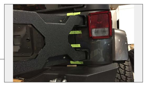
Install the tire carrier bracket to the hinges using the supplied hinge pins. Once installed, secure the hinge pins using the provided c-clips.
