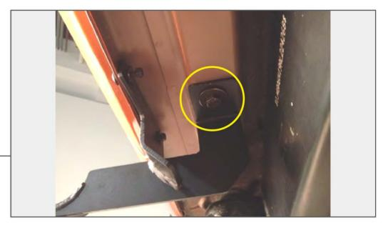
Insert (1) large bolt and (1) flat washer through the bracket and into the body hole that contains the nut plate. Hand tighten the hardware.
