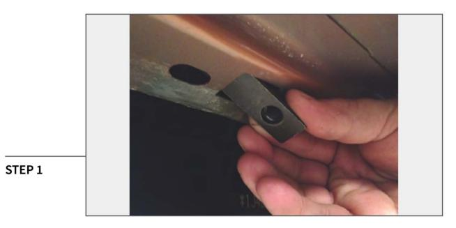
Insert (1) nut plate for each bracket into the existing holes on the bottom of the body.
