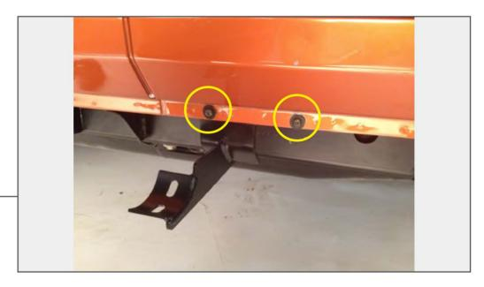
Place the correctly labeled bracket behind the pinch weld and loosely secure both holes with (1) hex head bolt and (1) flat washer placed through the pinch weld and bracket, then hand tighten with (1) flat washer and (1) nut on the inside.
