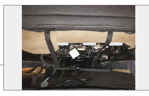
From underneath the seat, connect the front to back straps to the buckles. Pull tight on the strap to secure the cover to the lower seats.
