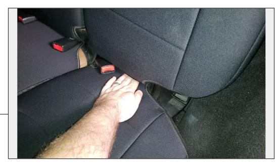
Insert the lower passenger and driver side seat covers. Tuck the buckles in-between the upper and lower seat section.
