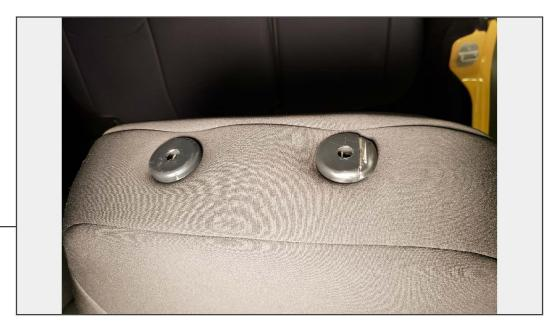
Once the upper portion of the seat cover is installed, tuck the seat cover under the tabs for the headrest guides.
