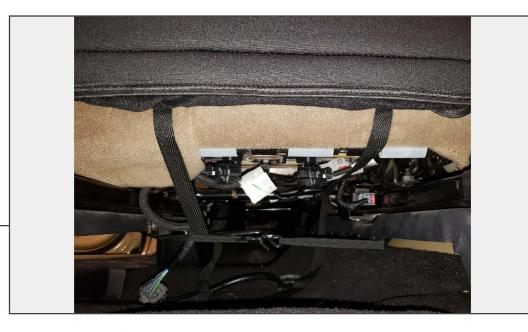
Connect the (2) front to back and (1) side to side clips to secure the seat cover to the lower portion of the seat. Then pull tight on the strap to ensure the seat cover is tight to the seat.
