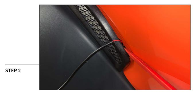
Using a plastic pry tool, pry back on the vehicle accent trim enough to insert the vent light wiring to the engine bay.
