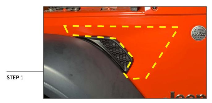
Clean the vehicle fender using the provided adhesion promoter pads along the indicated area.
