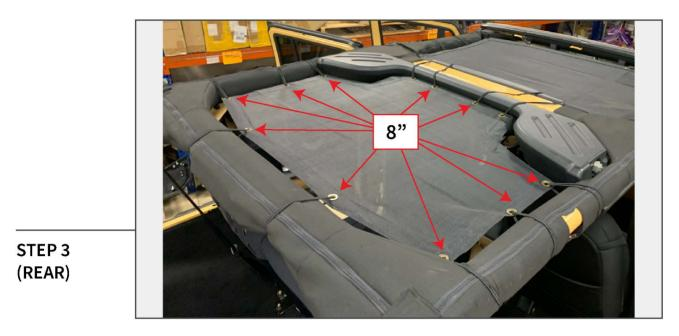
Using (10) 8" elastic bands, install the rear sun shade to the vehicle roll bars.
