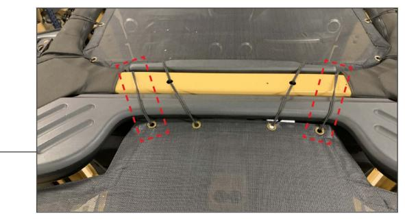
Using (2) 14" elastic bands, install the front inner corners of the mesh top to the vehicle roll bar.
