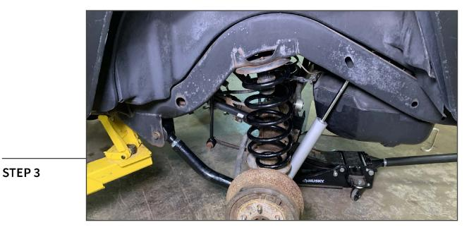
Fit the new shock absorber between the axle mount and the vehicle frame.
