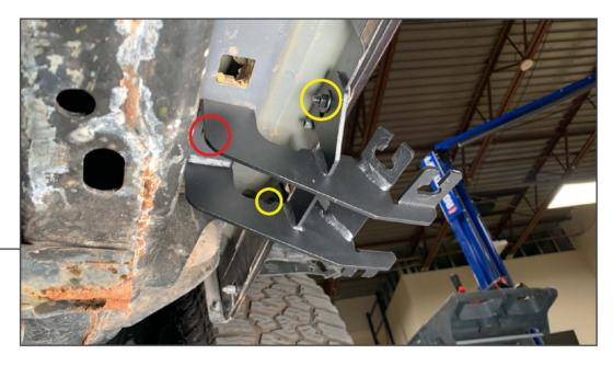
Secure the front mounting bracket to the pre-drilled holes in the vehicle using (1) M8x1.25 x 25mm bolt, (1) M8 lock washer, and (1) M8 flat washer. Secure the mounting bracket to pinch weld using (2) M6x1.00 x 25mm bolts, (2) M6 lock washers, (4) M6 flat washers, and (2) M6 nuts.
