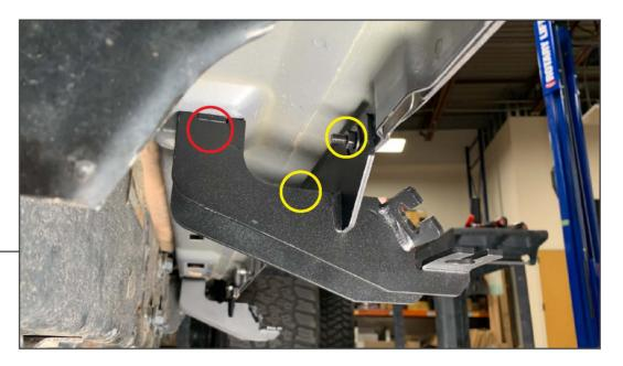
Secure the rear mounting bracket to the pre-drilled holes in the vehicle using (1) M8x1.25 x 25mm bolt, (1) M8 lock washer, and (1) M8 flat washer. Secure the mounting bracket to pinch weld using (2) M6x1.00 x 25mm bolts, (2) M6 lock washers, (4) M6 flat washers, and (2) M6 nuts.
