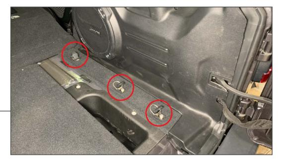
Remove (3) T-40 Torx screws to remove the (3) tie-down hooks from the cargo area.
