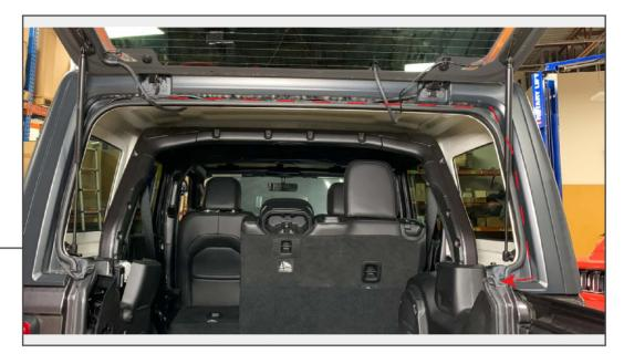
Clean the inside of the hard top with isopropyl alcohol and a microfiber cloth. Evenly space and adhere the wiring holders to the hard top. Insert the wiring harness towards the bottom of the hard top.
