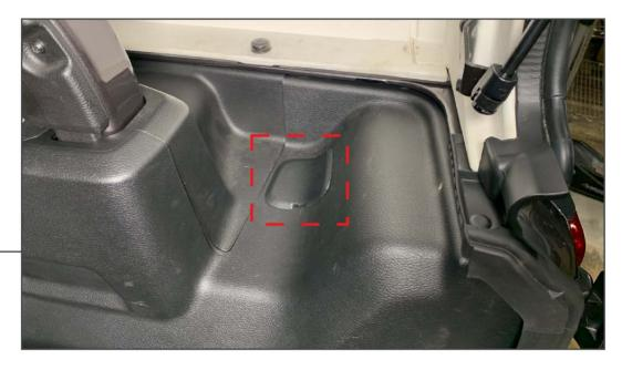
Remove the small plastic panel on the interior panel using a flathead screwdriver.
