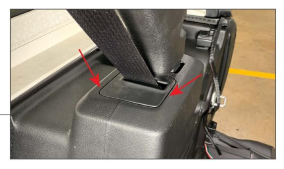
Using a flathead screwdriver, pry the seat belt plastic panel upwards to dislodge the panel.
