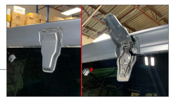
Pry upward on the bottom of the rear hinge cover using a flathead screwdriver. Once dislodged, hinge the hinge cover upward and push the cover upward to remove the cover from the vehicle.
