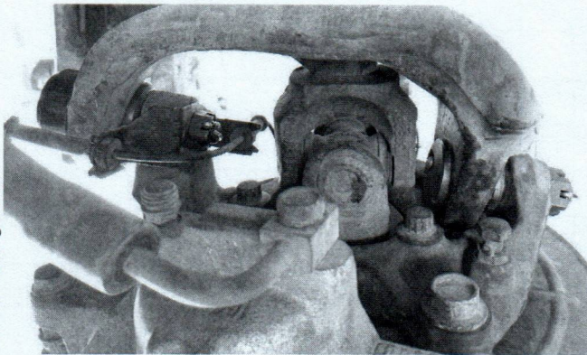
Figure 17. Finished Ball Joint Installation
