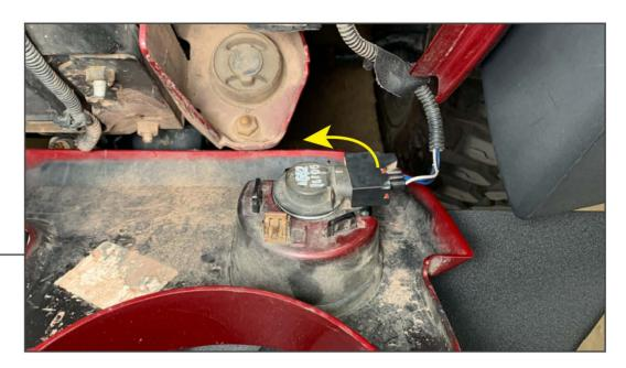
Twist the turn signal socket to remove the turn signal bulbs from the grille. Remove the grille from the vehicle.
