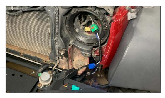
Plug the new headlight harness into the original vehicle headlight connector. Wire the DRL add-on harness following the diagram below.
