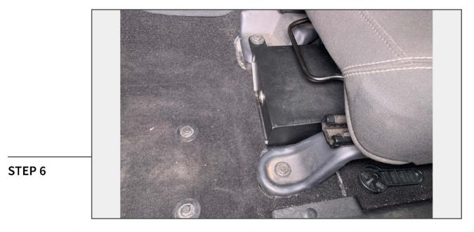
Re-install the (2) 18mm bolts into the seat brackets. Tighten each bolt to 45 ft-lbs.
