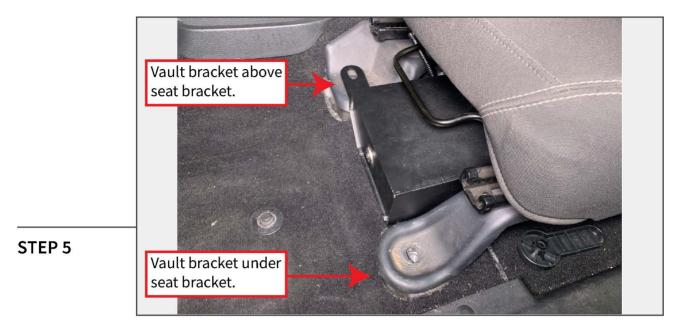
Insert the vault under the seat, ensuring the lower mounting bracket on the vault is under the seat bracket.
