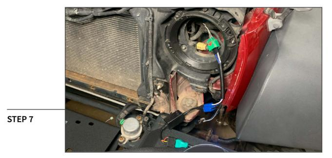
Plug the new headlight harness into the original vehicle headlight connector.
