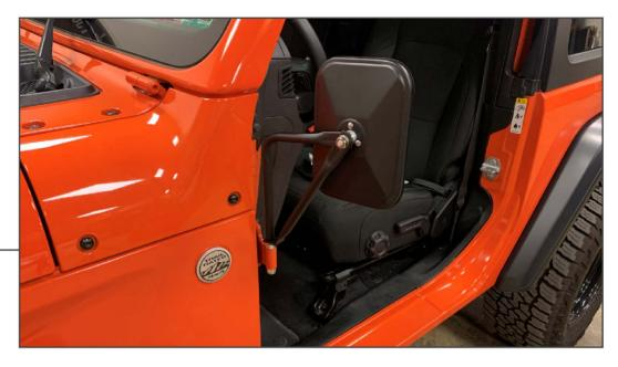
Install the mirror to the mirror assembly brackets using (1) M10 flat washer, (1) M10 lock washer, and (1) M10 nut. Tighten until secure.
