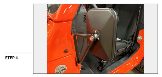
Adjust the mirror to the desired position, then tighten the (3) Phillips head screws to lock the mirror into place.
