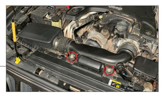
Open the hood. Remove (2) 10mm bolts from the top of the radiator assembly.
