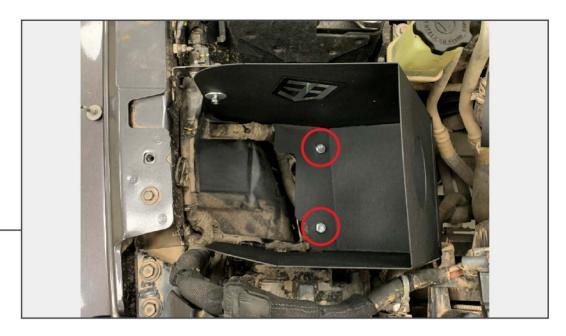
Insert (2) mounting studs into the original air box grommets. Place the intake heat shield over the studs, then insert (1) M8 bolt, (1) M8 lock washer, and (1) M8 flat washer through the heat shield into the mounting studs. Do not fully tighten hardware.
