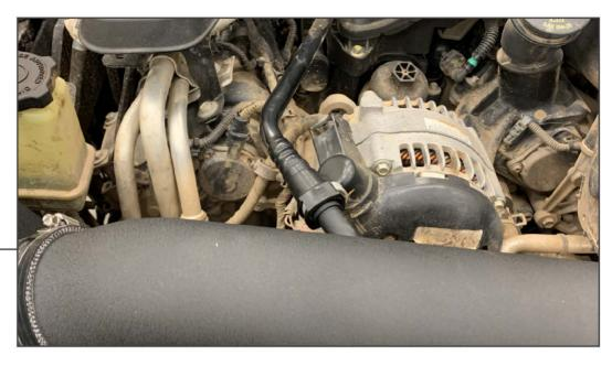
Install the PCV hose onto the intake tube. Press the tube until an audible click is heard, ensuring the tube is secured into place.
