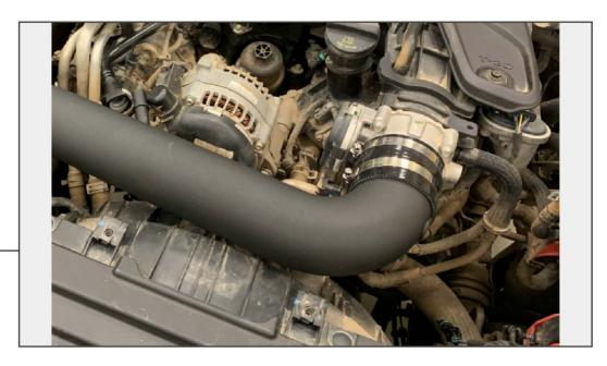
Use (1) coupler and (2) hose clamps to secure the intake tube to the throttle body. Do not fully tighten clamps.
