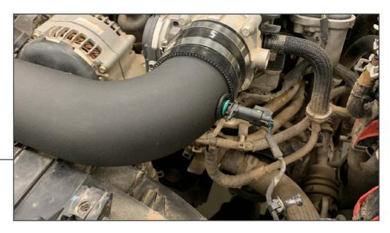
Install (1) sensor grommet into the hole in the intake tube. Press the temperature sensor into the grommet. Plug the wiring harness into the sensor.
