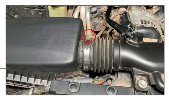
Loosen (1) hose clamp attaching the intake tube to the air box. Once loose, remove the intake tube from the vehicle.
