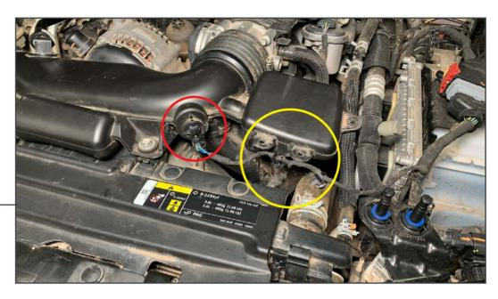
Unplug the intake air temperature sensor from the intake tube. Remove the (2) plastic hold downs from the intake tube baffle using a panel removal tool.
