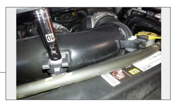
Remove the (2) 10mm bolts holding the intake to the fan shroud.
