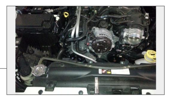
Pull the entire intake assembly up and away from the vehicle.
