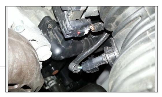
Unplug your factory IAT sensor located on the bottom of the intake tube.
