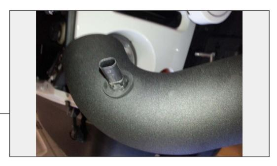
Remove of OEM IAT sensor and transfer it over to the new intake tube noting position.
