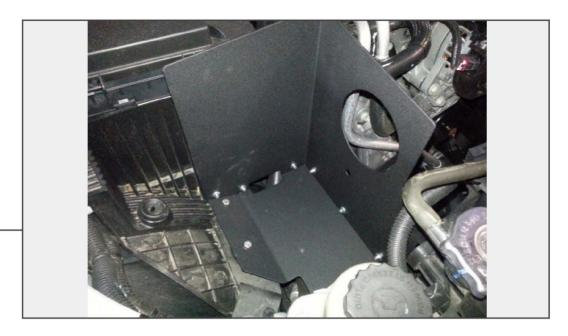
Install the heat shield using the factory mounting positions and secure with bolts.
