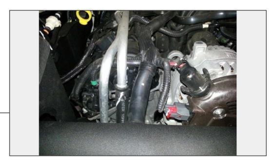
Reinstall the factory PCV hose onto the new intake tube and secure with new clamp.
