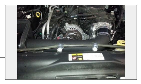
Using the supplied hose tie downs, re-secure the coolant overflow hose to the fan shroud.
