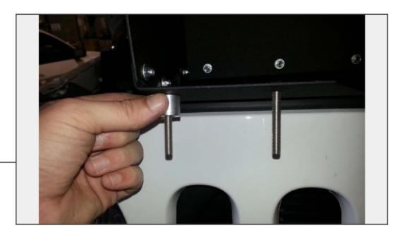
Add the supplied screws and spacers to the heat shield for mounting in the factory position.
