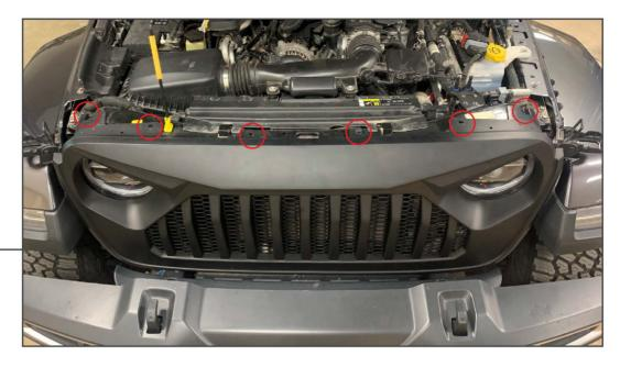
Align the bottom of the grille to the lower mounting bracket and clip into place. Hinge the grille up to align the upper portion of the grille to the radiator support. Insert (6) plastic push clips into the top of the grille.
