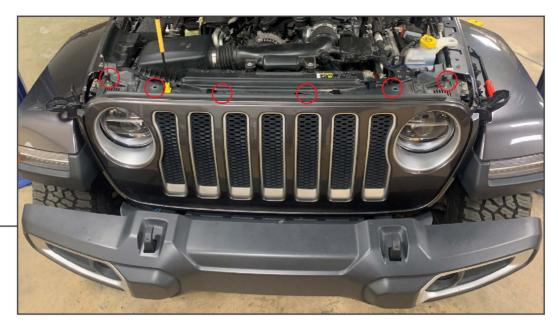
Remove (6) plastic push clips from the radiator support to release the upper portion of the grille assembly.
