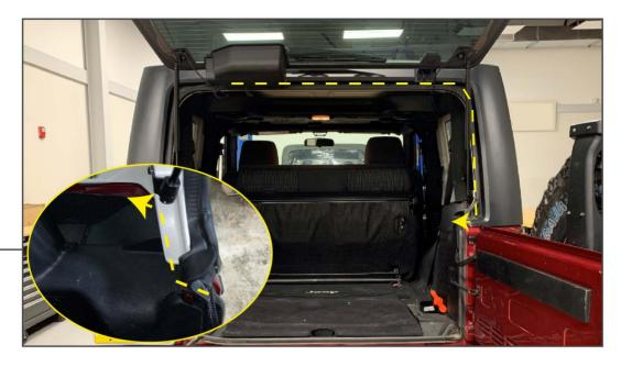
Using the (6) adhesive harness holders, route the wiring harness around the hard top weather seal. Route the harness under the gasket in between the tailgate and the hardtop into the interior.
