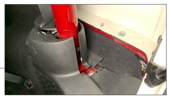
Carefully pry the trim panels apart. Remove the smaller panel to access the remaining 10mm nut.
