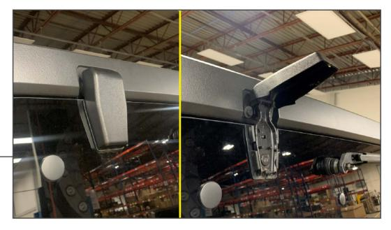
Using a plastic pry tool, gently pry the hinge covers from the rear glass hinges, starting from the bottom. The cover will hinge upward once dislodged. Lift the hinge cover from the vehicle.
