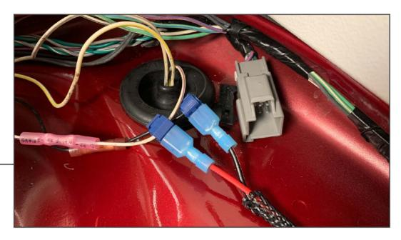
Splice the hinge lighting harness into the accessible vehicle wiring harness following the diagram below. Test each circuit before splicing. Use provided (4) scotchlok connectors to splice into wiring.
