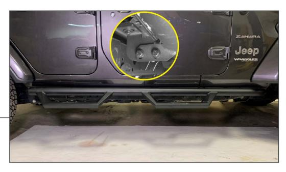
Install the tubular side step to the vehicle using (6) M10 bolts, (12) M10 flat washers, and (6) M10 locking nuts. Adjust the side step to the vehicle, then tighten all hardware until secure. Repeat steps 1-7 to the opposite side.
