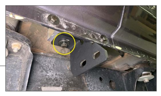
Install the rear pinch weld bracket to the vehicle. Loosely install (1) M8 bolt, (1) M8 lock washer, and (1) M8 flat washer through the pinch weld bracket into the pre-drilled hole in the vehicle.
