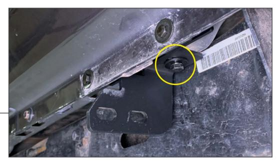
Install the front pinch weld bracket to the vehicle. Loosely install (1) M8 bolt, (1) M8 lock washer, and (1) M8 flat washer through the pinch weld bracket into the pre-drilled hole in the vehicle.
