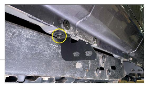
Install the middle pinch weld bracket to the vehicle. Loosely install (1) M8 bolt, (1) M8 lock washer, and (1) M8 flat washer through the pinch weld bracket into the pre-drilled hole in the vehicle.
