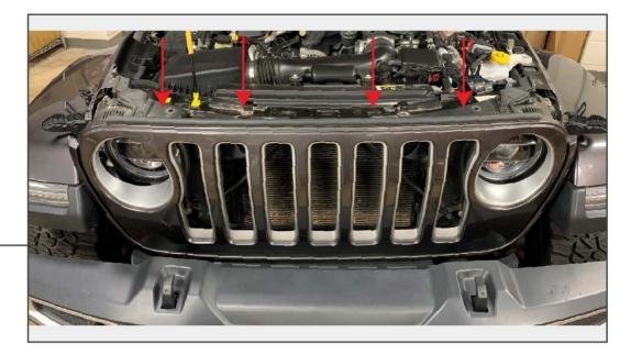
Loosely fit the grille to the vehicle. Place the grille insert in between the vehicle and the grille through the top.
