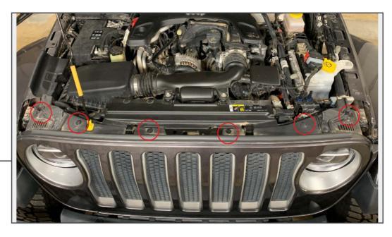
Remove the (6) push clips from the top of the grille.
