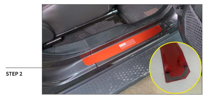
Peel the tape backing from the double sided tape. Align and apply the door sill guard to the vehicle. Firmly press down on the door sill guard to ensure proper adhesion. Repeat this procedure for the remaining door sill entry guards.
