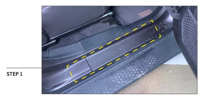
Clean the door sill with isopropyl alcohol and a microfiber cloth. Ensure the door sill is dry.
