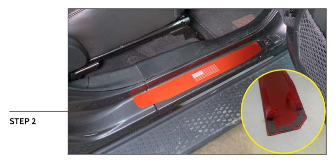
Peel the tape backing from the double sided tape. Align and apply the door sill guard to the vehicle. Firmly press down on the door sill guard to ensure proper adhesion. Repeat this procedure for the remaining door sill entry guard.
