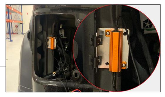
Using the provided clips, install the resistor and bracket onto the pinch weld behind the tail light.
