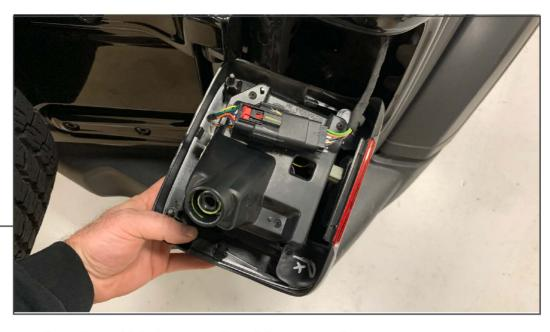
Pull the tail light away from the vehicle to access the wiring connection.
