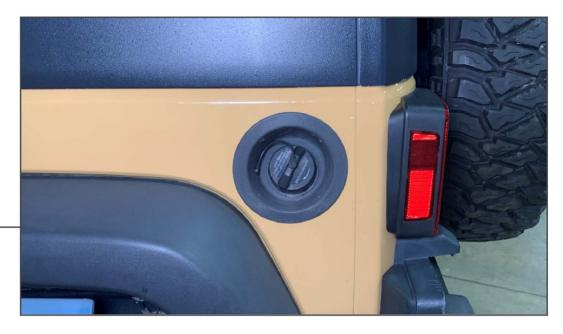
Clean the vehicle fuel tank trim using isopropyl alcohol and a microfiber cloth. Ensure the trim panel is dry.
