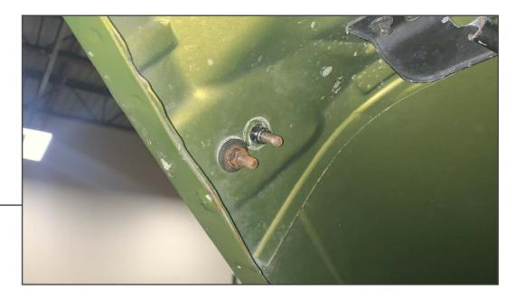
Open the hood on the vehicle. Remove (2) 10mm nuts from hood mounted portion of the latch system.
