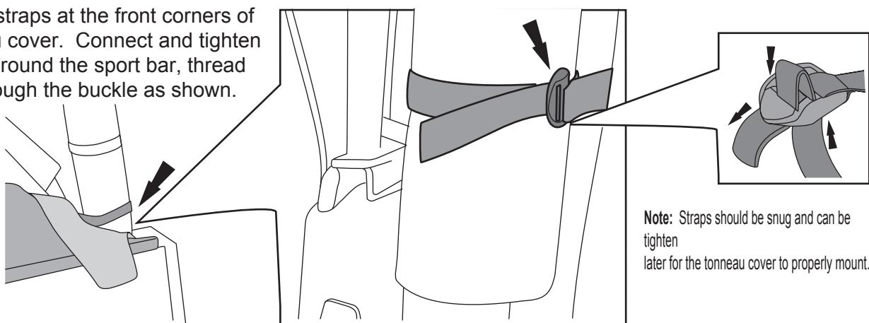
Note: Straps should be snug and can be tightened later for the tonneau cover to properly mount.
