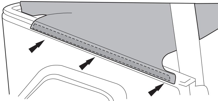
Tuck the plastic strip into the belt rail of the tub at the rear corners tailight area.
