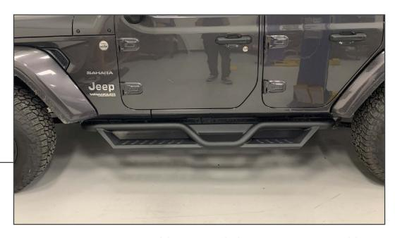
Install the drop side step bar to the vehicle using (6) M10 bolts, (12) M10 flat washers, and (6) M10 locking nuts. Adjust the side step bar to the vehicle, then tighten all hardware until secure. Repeat steps 1-3 to the opposite side.
