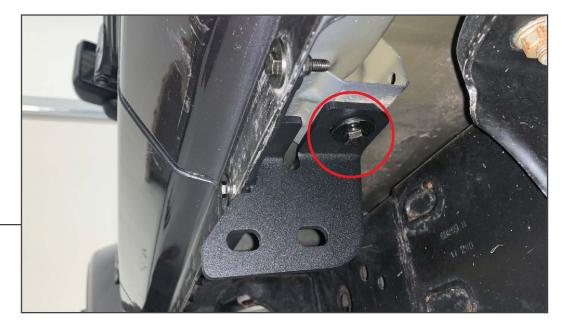
Install the rear pinch weld bracket to the vehicle. Loosely install (1) M8 bolt, (1) M8 lock washer, and (1) M8 flat washer through the pinch weld bracket into the pre-drilled hole in the vehicle.
