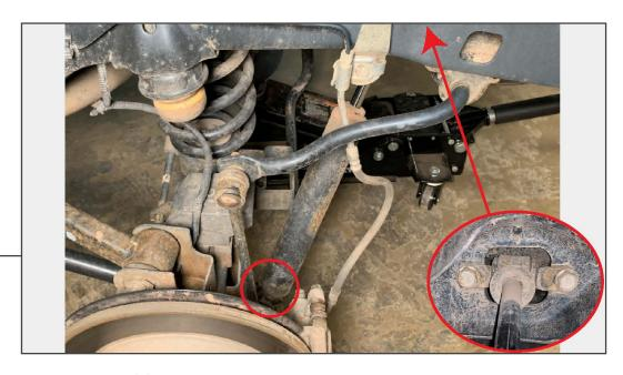
With the axle supported, remove (1) 18mm Nut and Bolt from the lower shock mount, then remove (2) 16mm Bolts securing the upper mount to the frame. Remove shock from the vehicle. Hardware will be reused. Repeat on both sides of vehicle.
