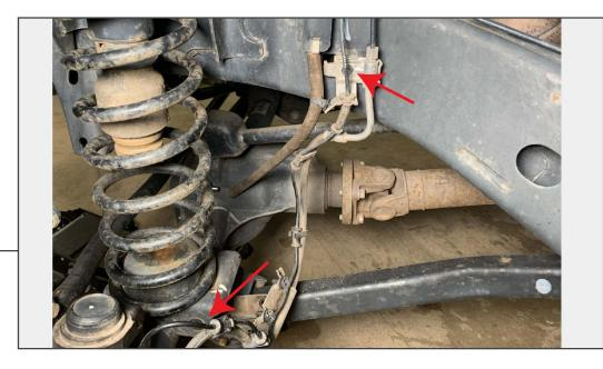
Remove the (2) 10mm bolts to release the brake line brackets from the vehicle. This will allow additional slack when lowering the axle.
