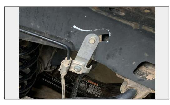
Gently massage the brake line to reach the bracket extension. Install the brake line extension to the brake line bracket. Bolt the extension to the frame using original hardware. Be sure the brake line is not touching anything.
