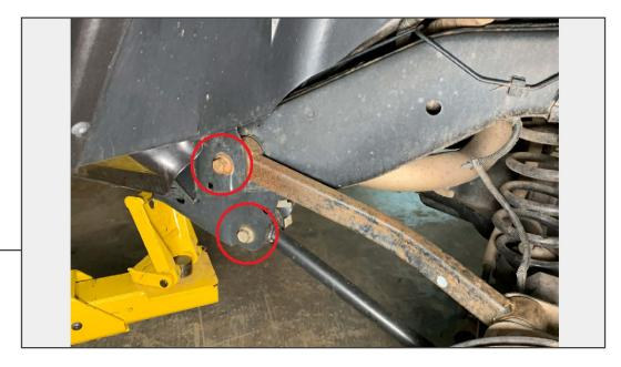
Reinstall the wheels onto the vehicle. While the suspension is loaded, tighten the control arm bolts attached to the frame to 125 ft. lbs.
