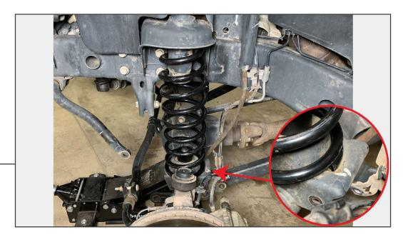
Install the new front spring (taller spring) onto the vehicle. Be sure to align the bottom of the spring with the cutout in the axle.
