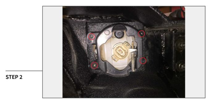
Locate the (4) factory screws, and remove. \*\*Note: Factory hardware will be reused.
