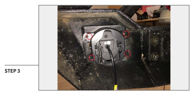
Install the new LED fog lights using the factory hardware.
