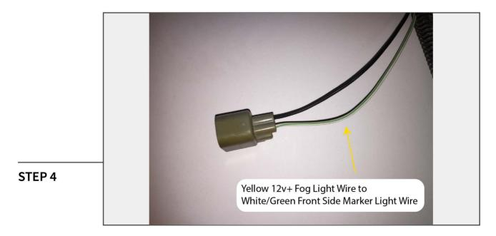
Splice the fog light into the vehicle's fog light harness. The additional yellow wire and blue wire will need to be spliced into the vehicle's factory wiring. Splice the yellow 12v+ fog light wire into the white/green front side marker light wire, then the blue wire into the vehicle turn signal harness.
