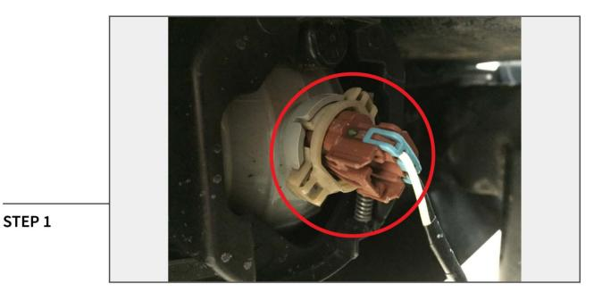
Access the connectors on the rear of the fog lights from the wheel well, and remove. \*\*Note: Light connector will be different between 07-09 and 10-18.
