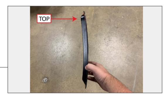
Familiarize the form of the grille inserts. The smaller end goes along the top of the grille. Test fit the inserts before removing the tape backing.
