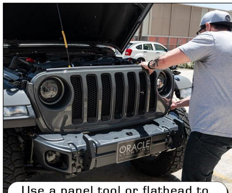
Use a panel tool or flathead to remove the retainer clips across the top. Firmly pull bottom of grill outward.
