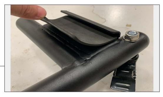
Install the (2) foam pads on each side frame by sliding it all the way to the back of the frame, and lay it down flat, firmly applying pressure to promote the adhesion.
