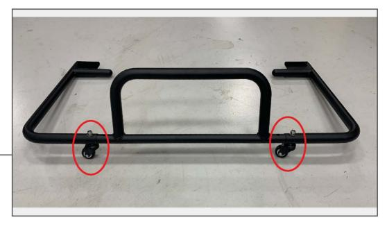
Install the (2) free casters at the appropriate alignment hole in the tube frames using (1) flat washer and (1) locking nut on each caster. Tighten the casters to the frame using a 17mm Socket, and hold the base of the caster stud with a thin wrench or needle nose pliers.
