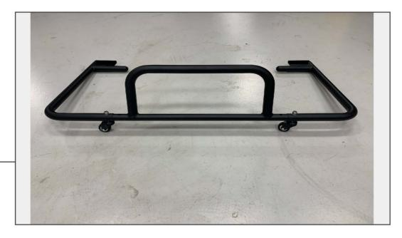
Lay out the front and the side frame tubes out to show similar to the picture above. Insert the side frame tubes into the front tube frame.
